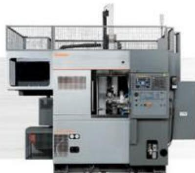
Sub-spindle equipped to complete products with front/back machining on a single machine
