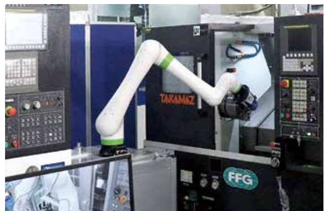
Example of use : HV-32A (FEELER) + CRX (FANUC, robot) + T-6i (LEADWELL)
