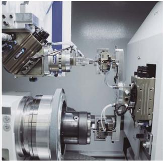
**BE- UND ENTLADEN MIT ROBOTER UND PALETTENSYSTEM**
